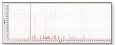
Figure 5. The powder diffraction pattern of atomoxetine hydrochloride produced through an ICDD Grant-in-Aid with collaborative agreement with X-ray Operations Research Division, Advance Photon Source, Argonne National Laboratory, to be published in Powder Diffraction.
