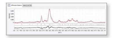
Figure 2. Experimental data (red) compared to a simulated hydroxyapatite of 90 Å crystallite size and oriented along [100] (grey).
