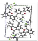
Figure 4. Unit cell and molecular structure for atomoxetine hydrochloride. The structure was solved and refined using synchrotron powder diffraction data, and Rietveld and density functional techniques.
