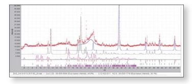
Figure 1. The diffraction pattern (red) from a crushed tablet of Lipitor<sup>®</sup>. The digital patterns underneath are the digital patterns of the ingredients identified from the PDF-4/Organics database.
