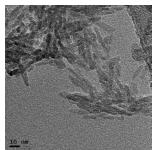
Figure 4. Photo of nano-apatite. Photo and specimen courtesy of Transparent Materials, LLC.
