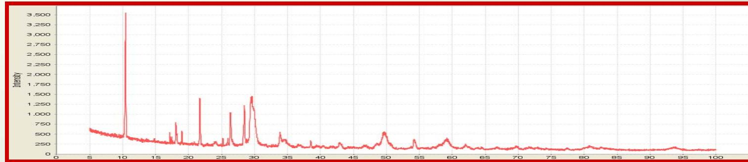
This is the diffraction pattern taken from a specimen of a catalytic converter. In this tutorial, this pattern will be extensively analyzed.
