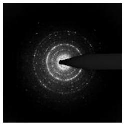
Pawley and Rietveld refinements using electron diffraction from L1<sub>2</sub>-type intermetallic Au<sub>3</sub>Fe<sub>1-x</sub> nanocrystals duringtheir in-situ order–disorder transition
