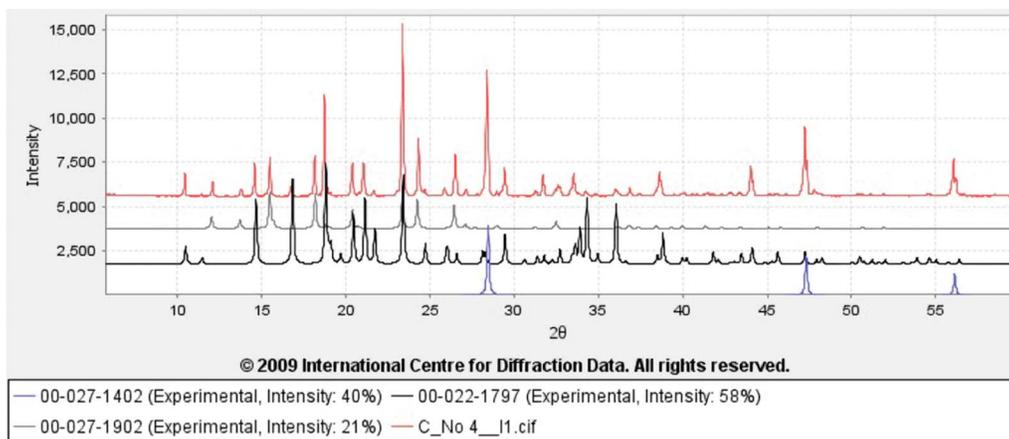
Figure 2. (Color online) Phase identification of the three component mix. The experimental data are shown as the top scan and the three identified phases are shown as digital simulations in the three scans below the top scan. In these data the doublet centered around  $18^\circ 2\theta$  (Cu) in the top scan has a contribution from each of the two major pharmaceutical phases shown in the next two scans.
