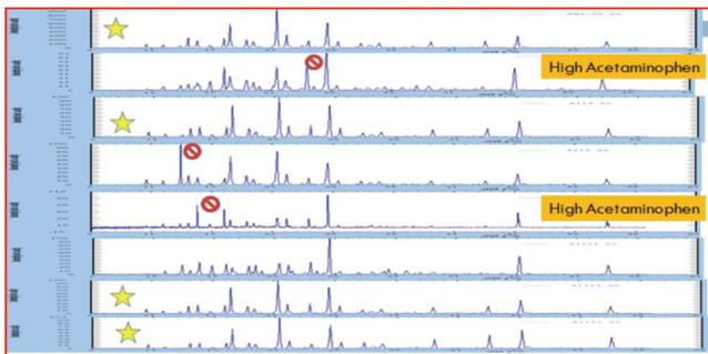
Figure 1. (Color online) Raw data from eight laboratories placed on similar scales for the three component mixture of acetaminophen, mannitol, and silicon.
