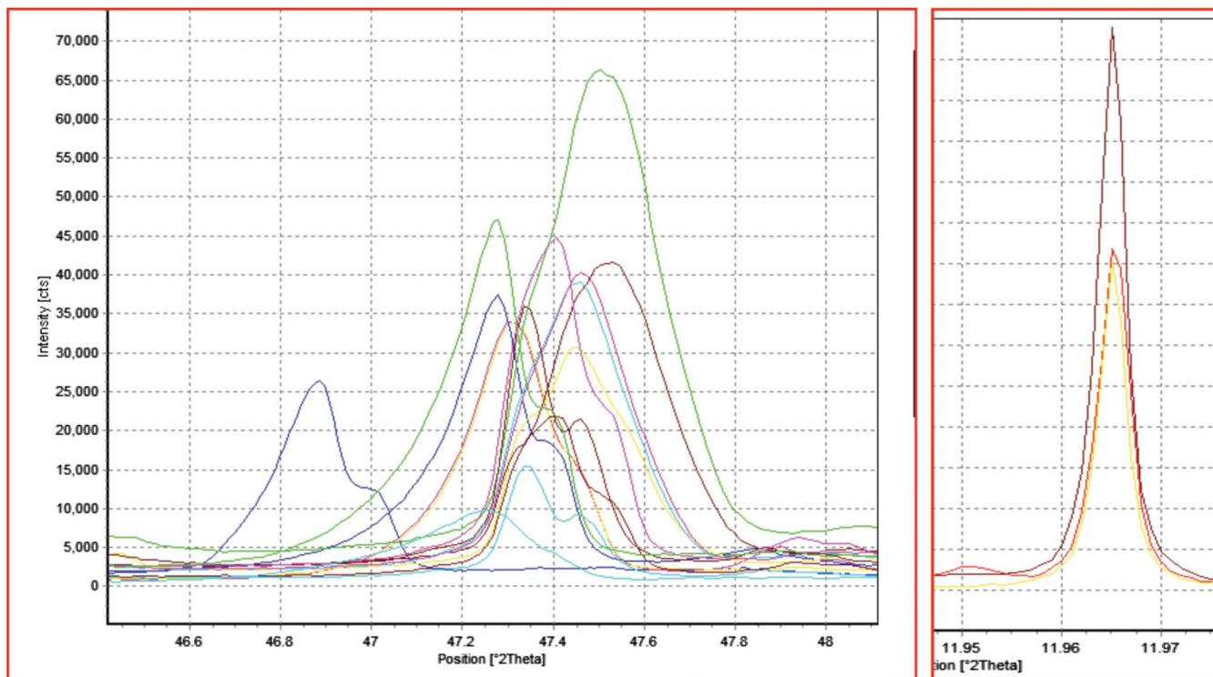
Figure 7. (Color online) Multiple data scans from round robin participants showing the 220 reflection of silicon; displacement errors are evident from the wide range of positions. NIST SRM 640c was the source of silicon. For comparison the same reflection is shown using monochromatic radiation taken at the ESRF where one can see the significant improvement in resolution.
