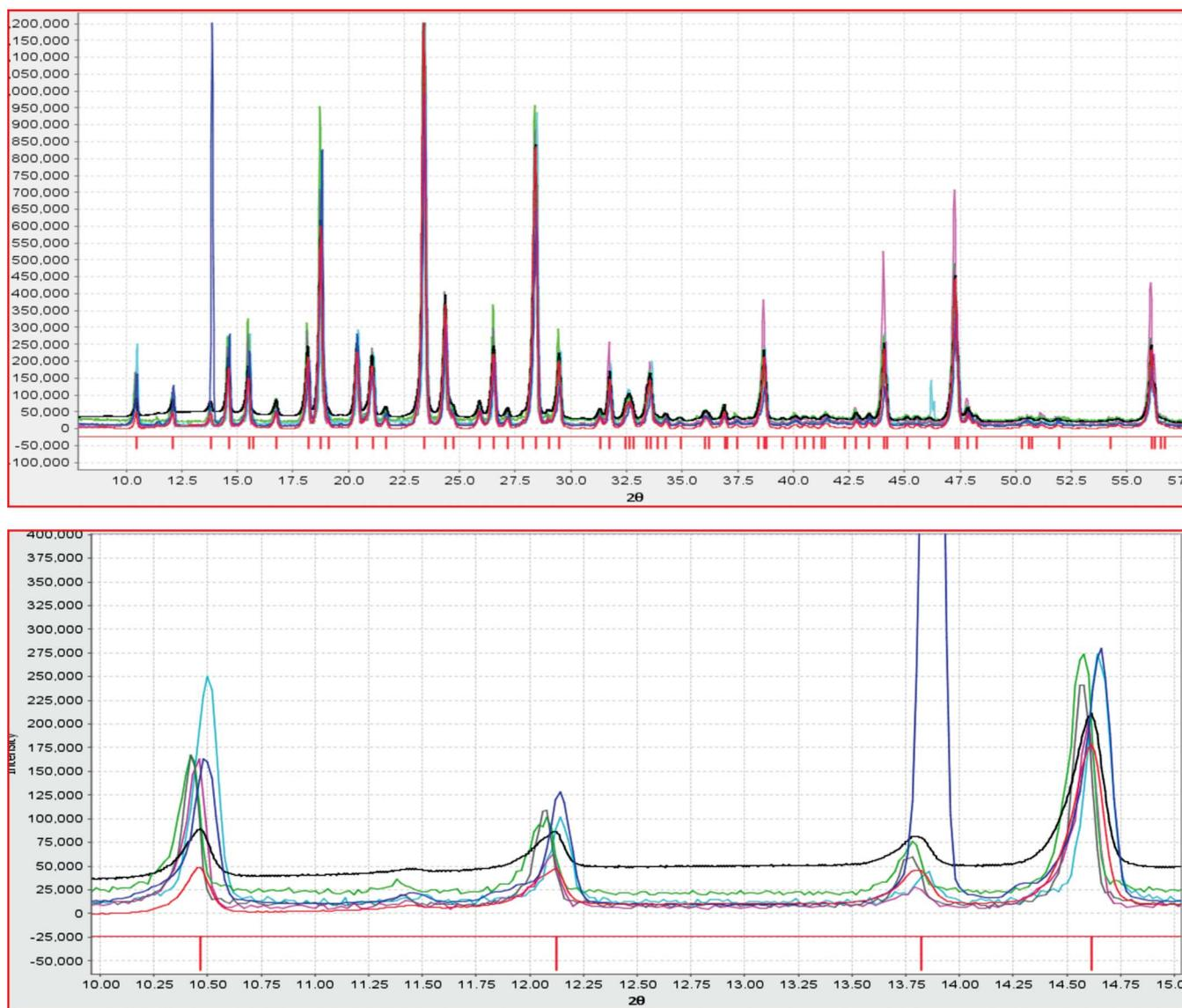
Figure 8. (Color online) (a) Superimposed data from seven laboratories for the three component mixture that were all scaled to the maximum peak. (b) Data from seven laboratories are superimposed for the three component mix. The outside two peaks are due to mannitol and the inside two peaks to acetaminophen. The off-scale peak is characteristic of severely oriented acetaminophen.
