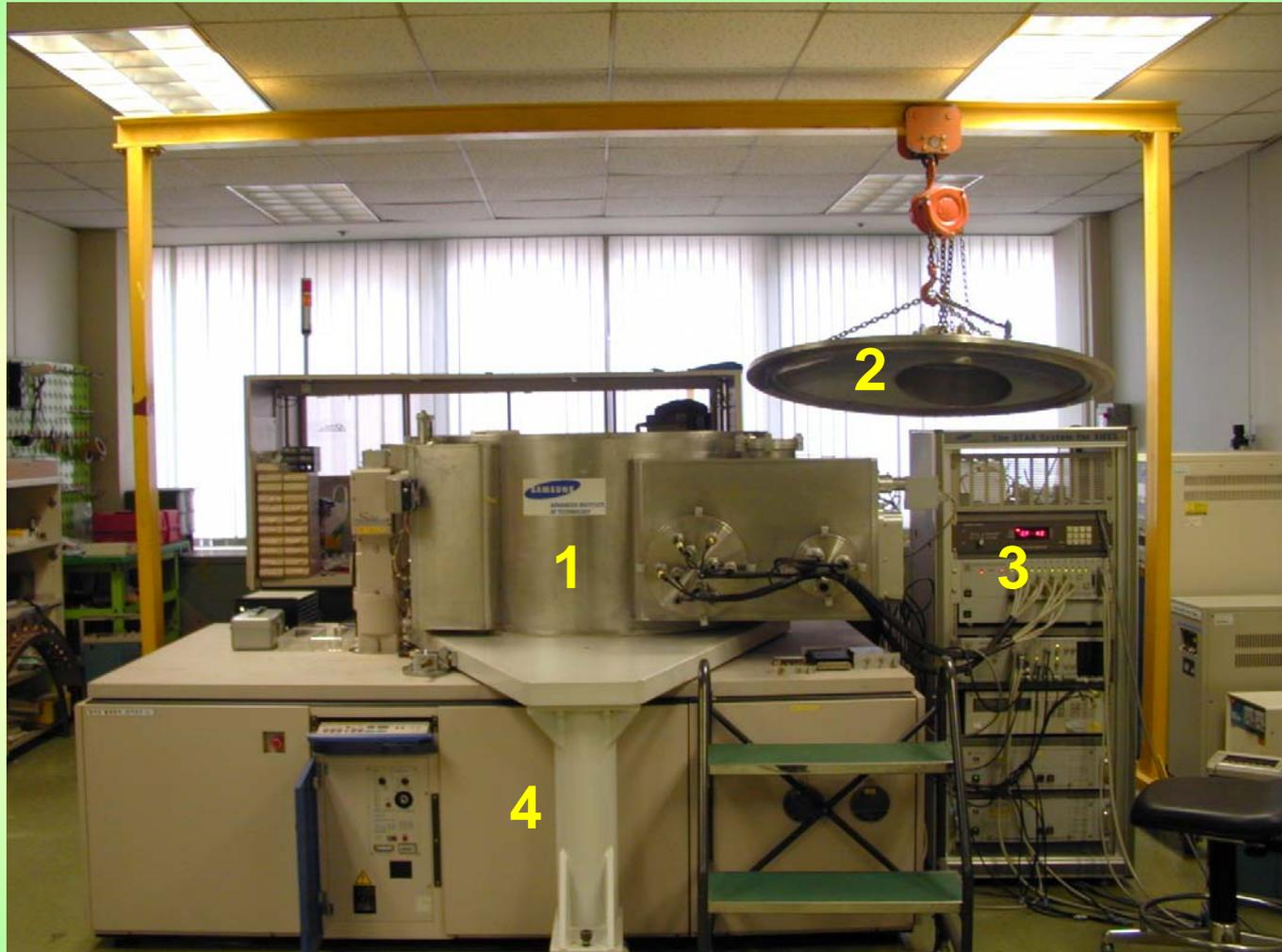
1 is the vacuum spectrometer chamber (dia. 1300 mm), 2 is the cap hung on telfer, 3 is the registration system, 4 is the x-ray rotating anode source. The total device weight is about 2 tons.
