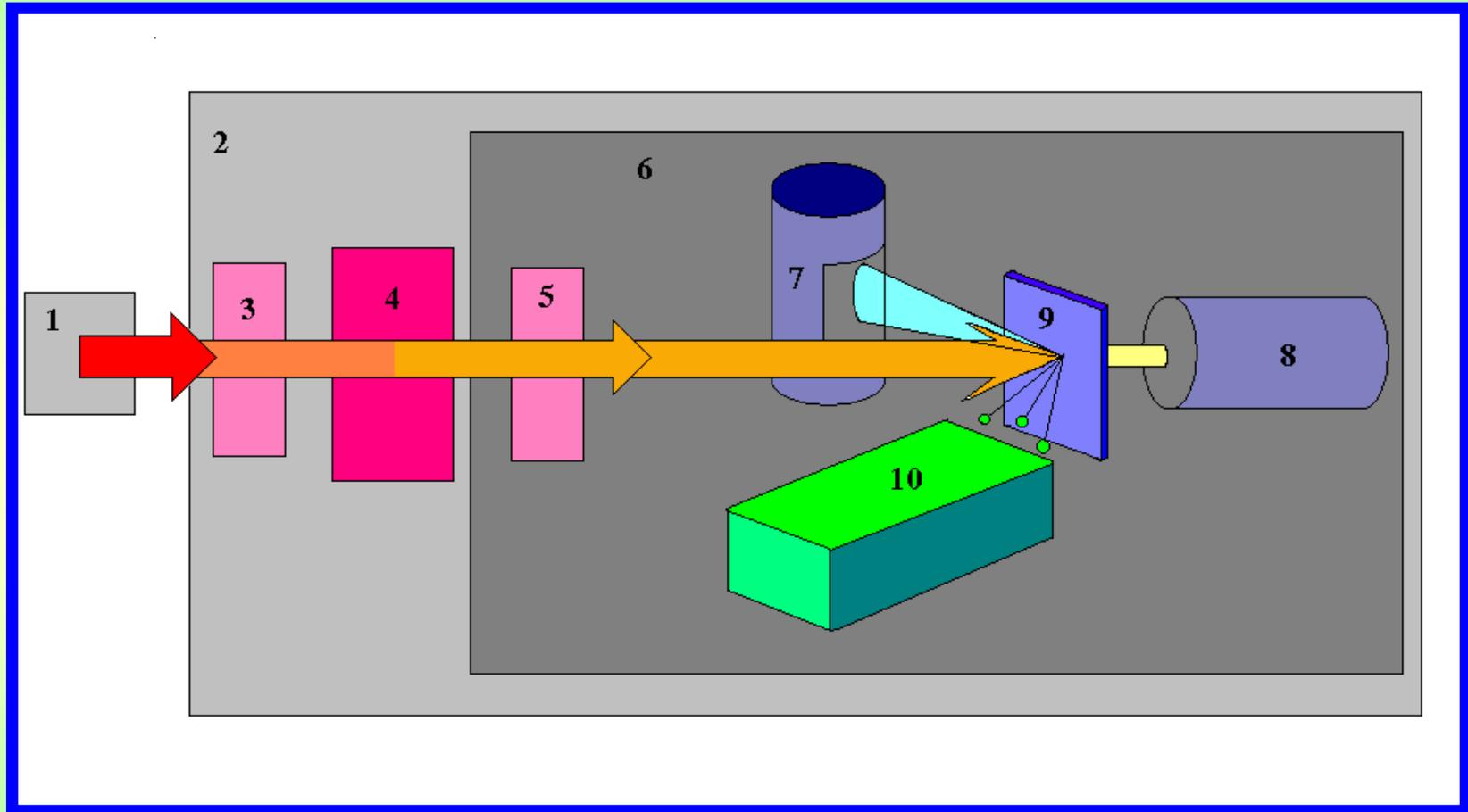
1 - X-ray generator, 2 - spectrometer vacuum volume, 3 - entrance slit,
