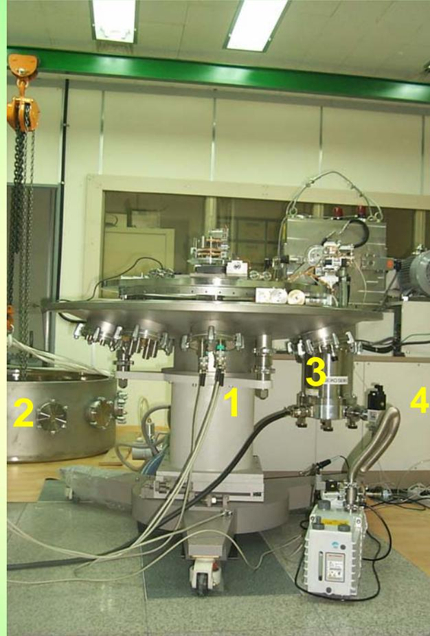
1 is the vacuum chamber exposed to the atmosphere, 2 is the wall of vacuum chamber with technological flanges, 3 is the turbomolecular vacuum pump STP 1003, 4 is the x-ray rotating anode source with the power up to 60 kW. The chamber diameter is 1300 mm, the total device weight is about 1.5 tons.
