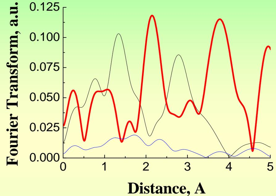
The bold red curve is related to ceruloplasmin, the black curve describes Cu<sub>2</sub>O, and the blue curve corresponds to Cu(NO<sub>3</sub>)<sub>2</sub>·3H<sub>2</sub>O.
