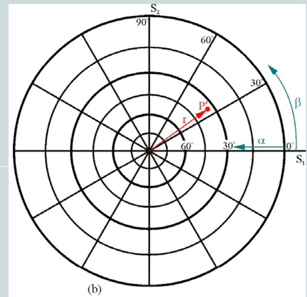
The pole figure angles ( $\alpha, \beta$ ) can be calculated from the unit vector components by the pole mapping equations:
