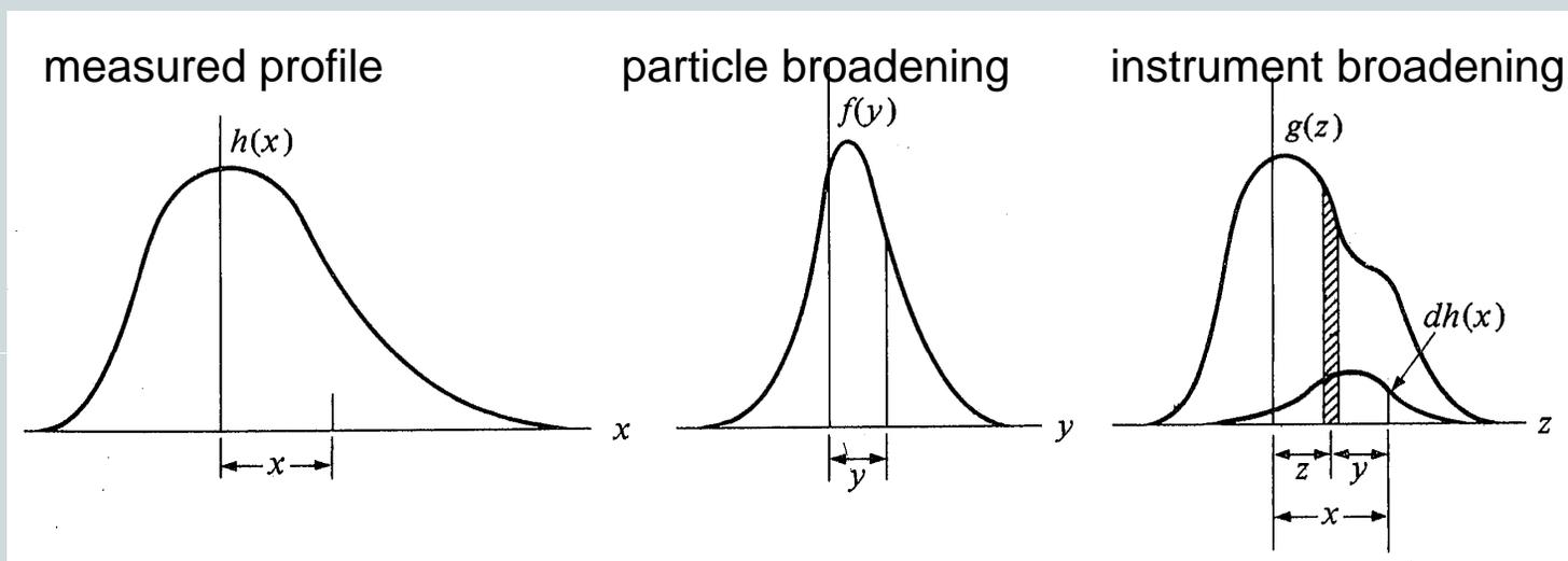
The measured profile is a convolution of the functions representing particle-size broadening and instrument broadening
