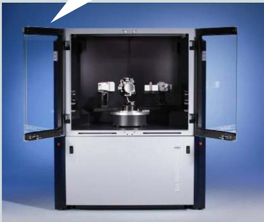
Sliding door: easy access for sample loading and configuration changes
