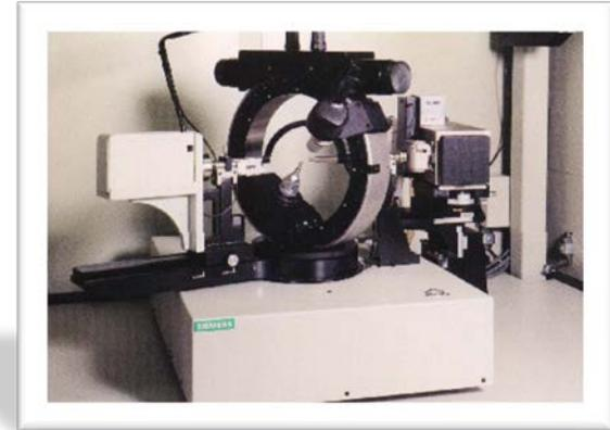
By tilting the TEM goniometer (single /double tilt, tilt rotation , tomography) we can reconstruct the reciprocal space of the crystal . Tilt angle may vary from  $-70$  to  $+70$  deg or less depending on TEM configuration and TEM goniometer specifications
