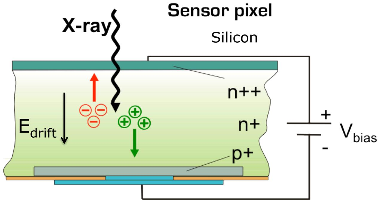
Interaction of X-rays and Si produces charge. Charge drifts through the sensor.
