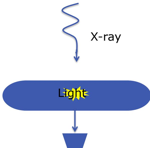
Indirect detection of X-rays
