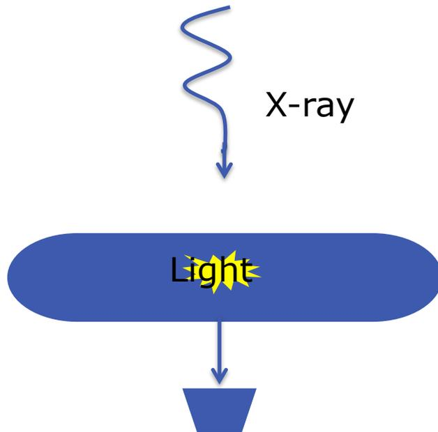
Indirect detection of X-rays
