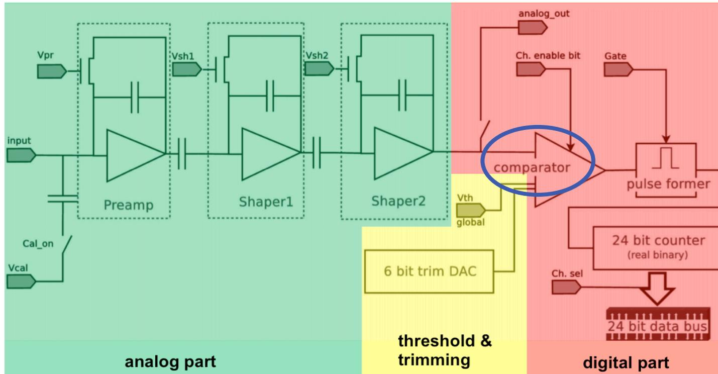
Signals with Energy higher than the threshold are accepted for counting.
