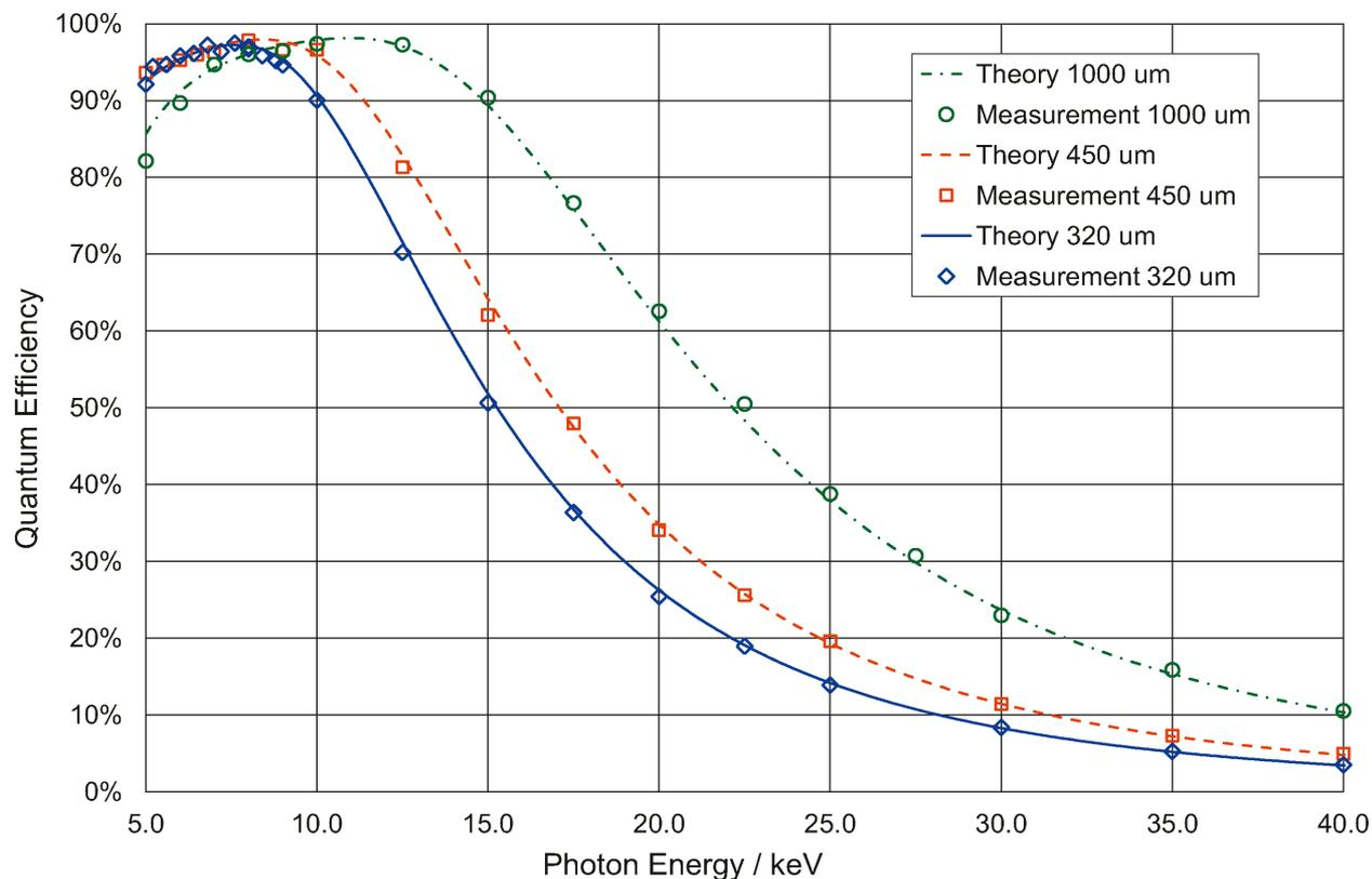
Efficiency of the silicon sensor depends on its thickness and X-ray energy.
