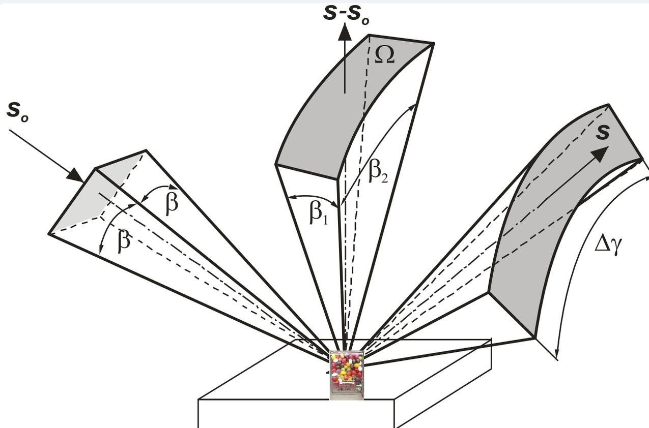
For XRD<sup>2</sup>, the instrumental window  $\Omega$  is given by
