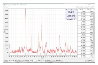
Figure 1: Graphical display of analysis of opal base, using PreDICT.
