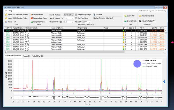
Experimental data that was imported and processed in JADE, can now be imported into Sleve+ for complimentary phase identification.
