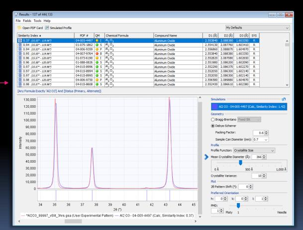
Quick settings panel allows the user to dynamically change various simulation settings directly on the graph.
