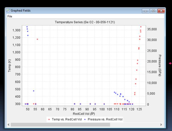
Temperature series graph for Ge O2 displaying both temperature (left y-axis) and pressure (right y-axis) as a function of reduced cell volume.\*
