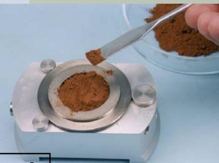
If the mineral is soft an agate mortar and pestle can be used to produce a fine powder. If the mineral is hard mechanical grinding may be required.
