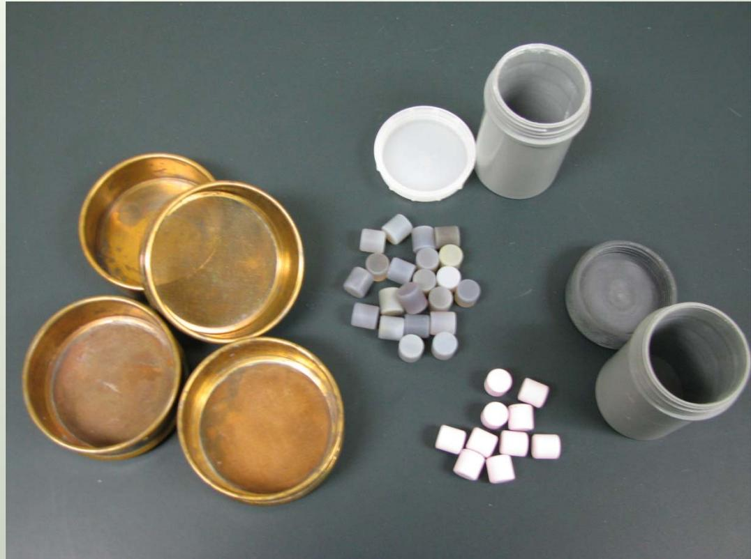
On left: Particle sieves of 100, 200 and 600 mesh
