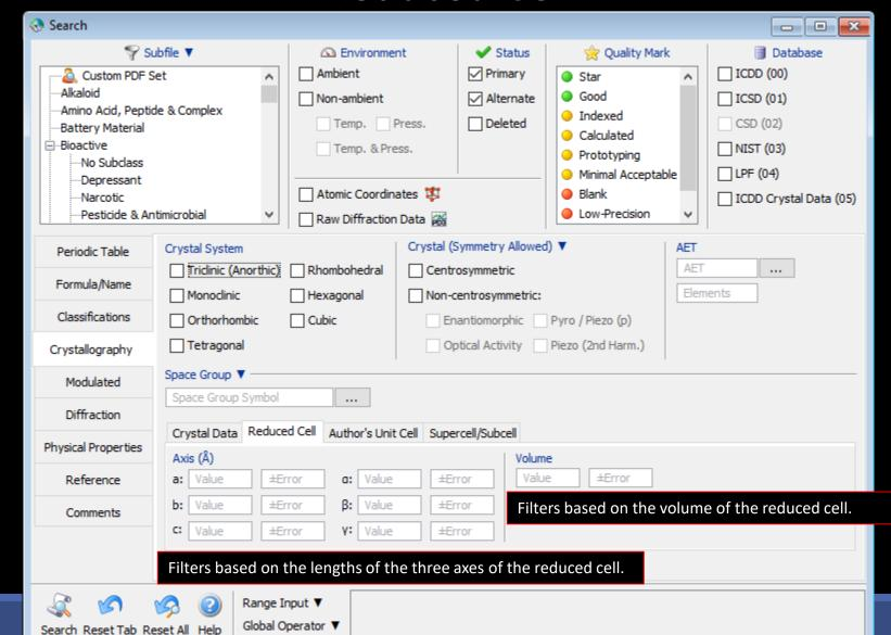
The reduced cell is a unique, primitive cell based on the three shortest lattice translations.
